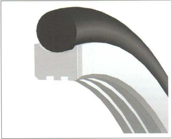
Fig. 5. New trunnion composite seal design.
